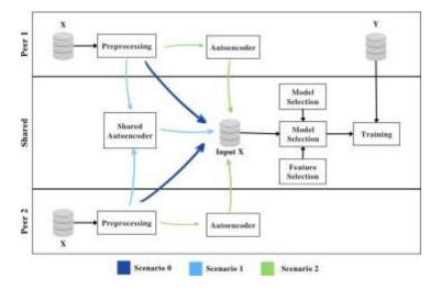
Figure 2: General Autoencoder Structure for Training Phase and Explored Scenarios
